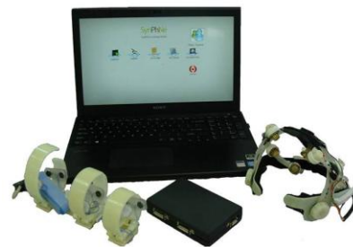
Fig.1. The system consists of a data capture unit (black box) which has two connectors, one each for EMG and EEG inputs from armgear and headgear shown to left and right side of the black box respectively.
