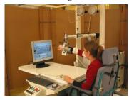
Figure 2. The Gentle/s System – Can be converted to HMHI with 2 chairs, 2 guides and common controls.
